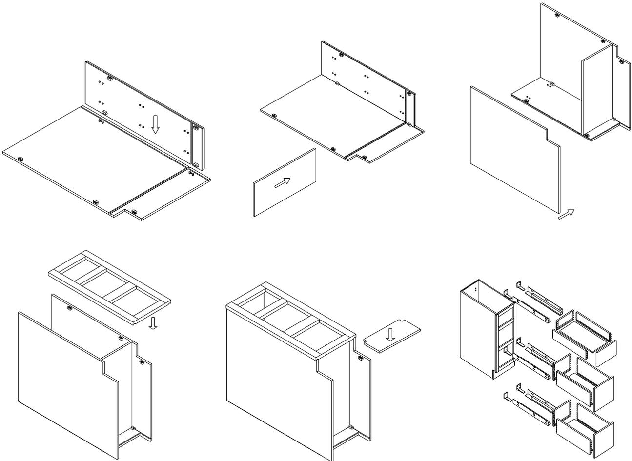
1. First put the grey rail holders into the holes on the back panel. Then lock the back panel onto a side panel.
