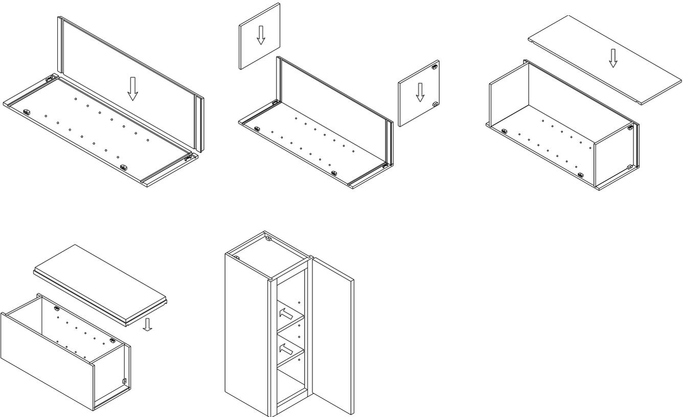
1. Put the back panel in the back groove on one of the side panels.
