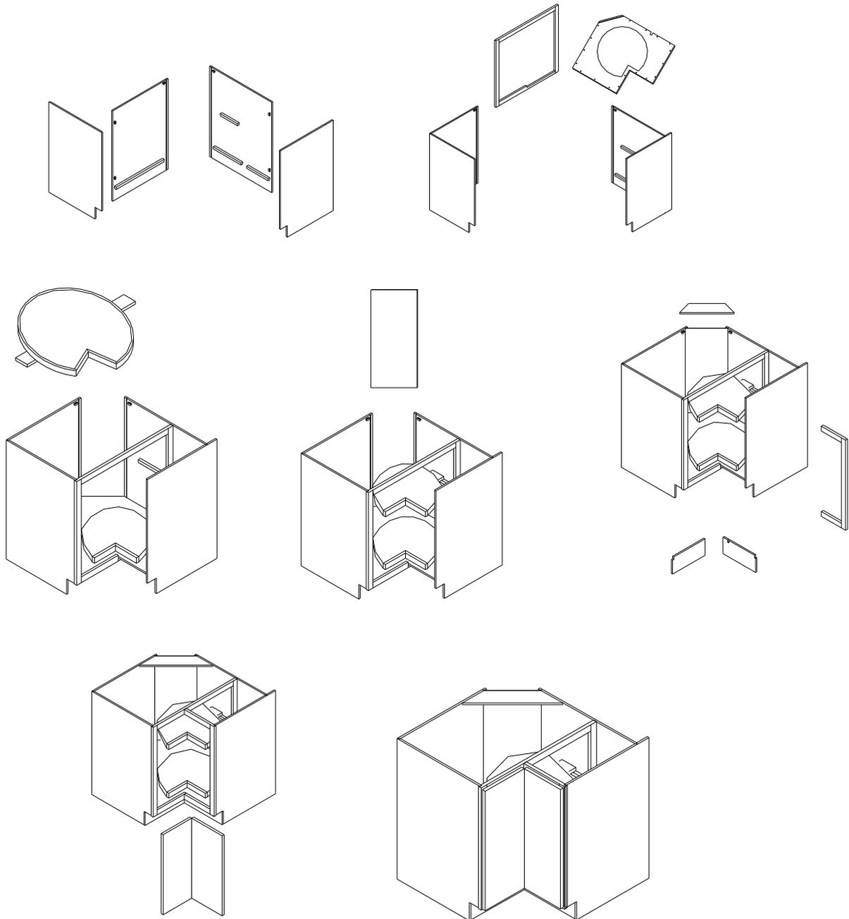
First lock the side panels together. The wooden piece attached to the side panels should be at the bottom for all the panels.
