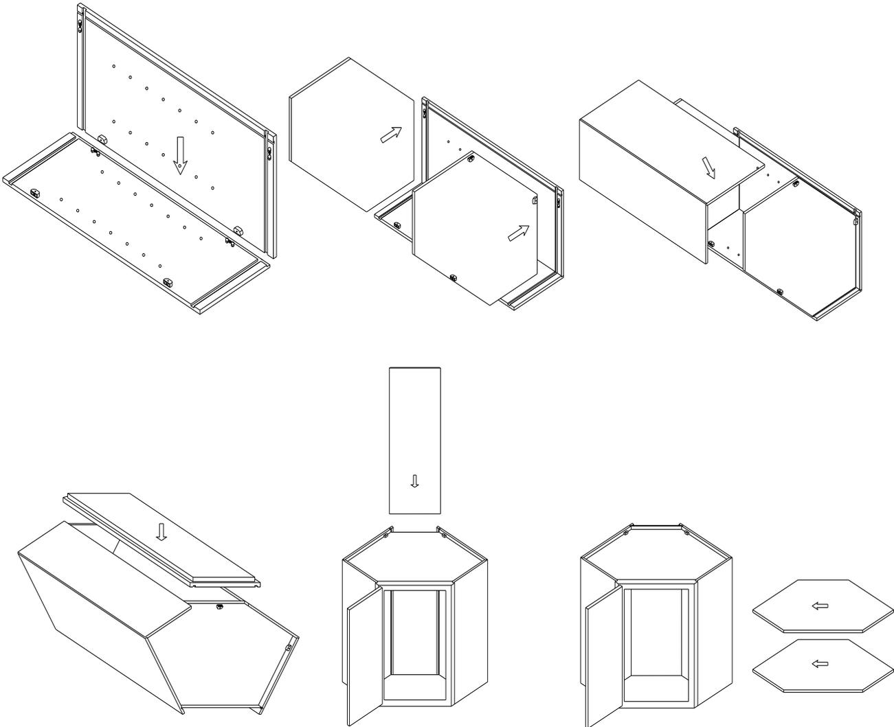
1. Line up the grooves of the side panels, 1 wide one and one narrow one. Make sure all the cam locks are open. Lock the two sets of side panels together.
