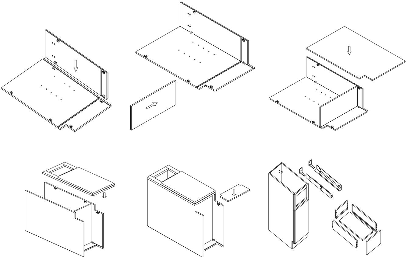
1. First put the grey rail holders into the holes on the back panel. Then lock the back panel onto a side panel.
